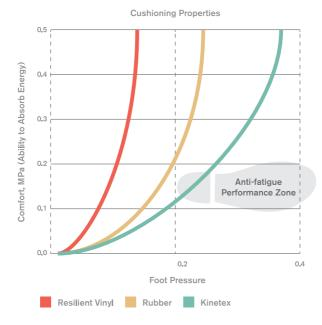
Source: Conducted by an Independent Testing Laboratory
